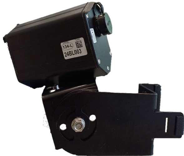
Figure 14 : installation for stop-line detection, radar on the right in the direction of travel 20° vertical/-30° horizontal
