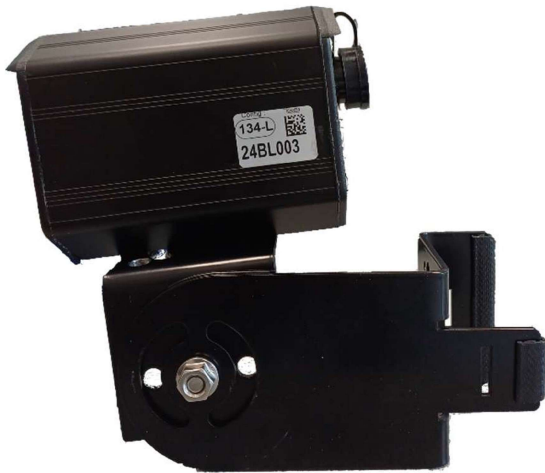
Figure 13 : distant detection installation < 5° vertical/0° horizontal
