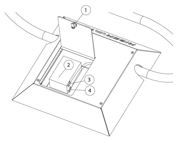
When the battery has reached a level of charge is too low to adequately perform the lifting and lowering of the bow, the control unit will bring the bow down position and will stop accepting additional radio commands.
