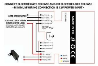
Do not use the shown wiring for an electric lock if it needs more than 300mA. Use separate power source. For gates & barriers connect as shown on output 1.
