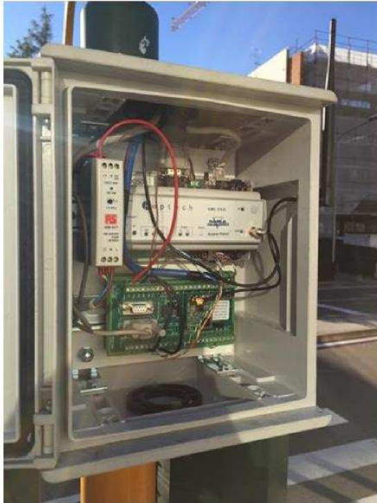
Fig. 2.2. TDM WI - Hub, T.L.I.C. & Access Point installation
